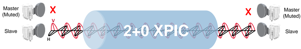
Figure 38: MIMO Resiliency – Slave Unit Half-Capacity Link
