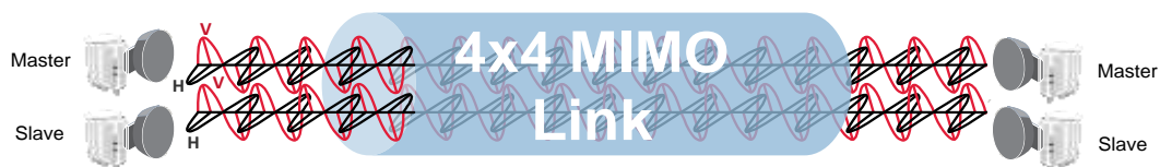
Figure 36: 4x4 MIMO Configuration – Master and Slave Units
