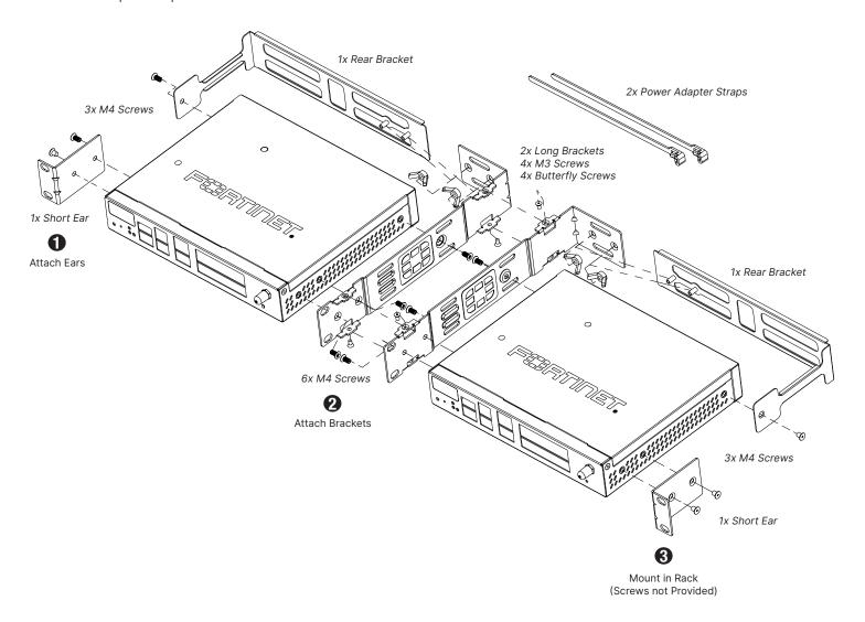
Note: The recommended clearance is 1.5 inches above and below the device.
